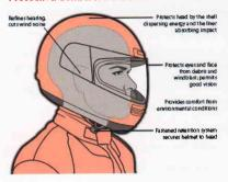
padding; and a good retention system. What we see first is the outer shell, usually made from some family of fiber-reinforced composites or thermoplastics like polycarbonate.
